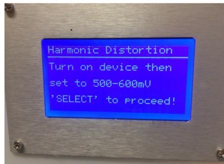
3. Press 'SELECT' again to proceed test signal calibration, set output level to around 500mV-600mV
