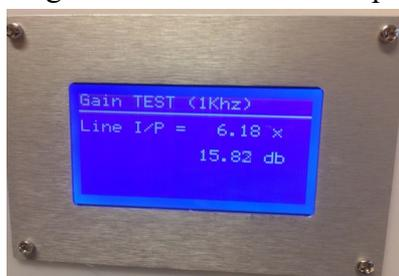
5. If the DUT is a stereo unit, then remove the channel just been tested and connect to other channel, the gain reading of the other channel will show right away.
