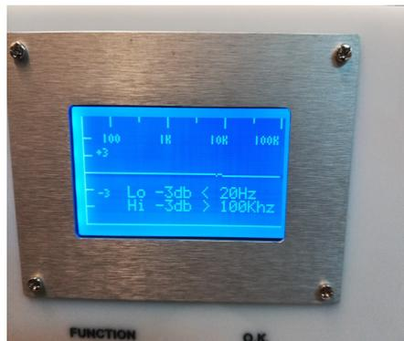
You will be able to observe a frequency response curve as follow, and the tester will tell you the low and high -3db point frequency of the DUT. If the high -3db point is higher than 100Khz, then it will simply shows "Hi-3db > 100Khz". If the low -3db point is lower than 10Hz then it will simply show "Lo-3db < 10Hz"
