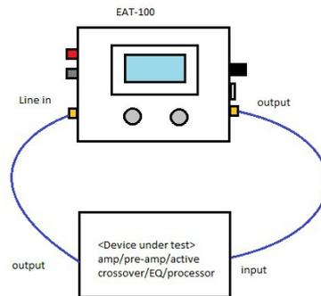
For power amp or integrated amp connect as follow, set input selector of the tester to 'speaker level' :
