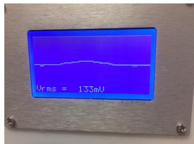
4. Set the DUT to max. volume / gain . Press 'SELECT' to proceed and view the test result.
