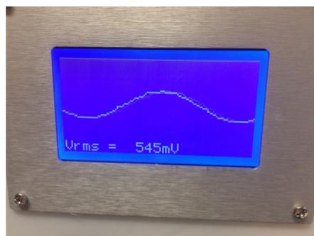
4. Press 'SELECT' to proceed and view the test result. The following is an example of heavily distorted output from DUT with lots of odd harmonics.
