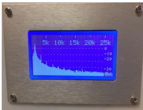
Press “FUNCTION” during testing can change the vertical scale between 5db / 10db
