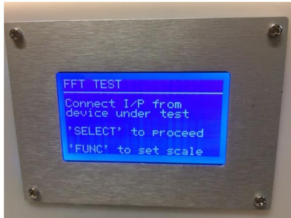
3. Connect from DUT to the input (line level or speaker level) , then press 'SELECT' once more to proceed the testing
