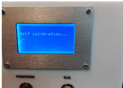
7. There will be self calibration before actual testing for max. accuracy
