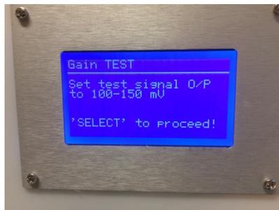
3. Press 'SELECT' again to proceed test signal calibration, set output level to around 100mV-150mV
